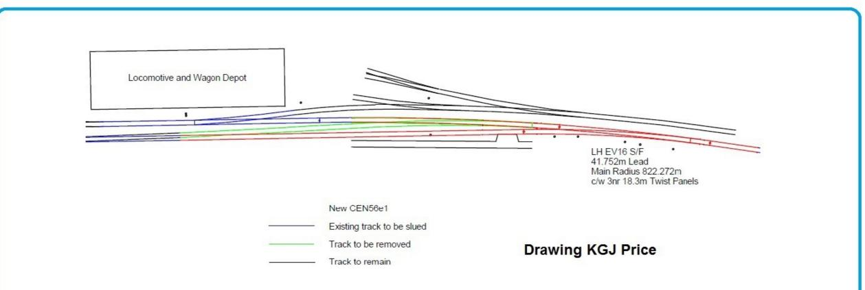
Repositioning points 12B away from the station will improve the alignment and enable the platform to be extended.
