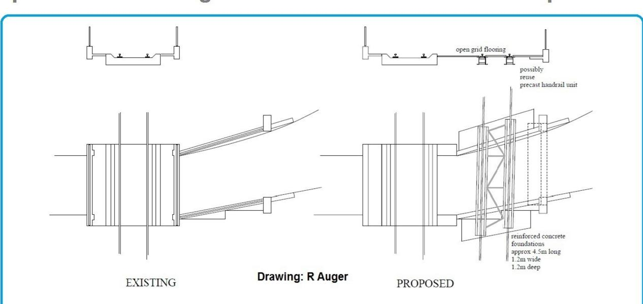
The new bridge will not restrict stream flow and will allow future flood water to filter back into the stream.
