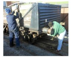
ends and metalwork has been painted olive, which is the correct livery, rather than black. Planks to replace those too rotten to repair will be along soon as they are being tanalised. The existing woodwork has been coated with 2 pack epoxy primer. 46253 lags behind a little but is now rubbed down and the headstocks painted matt black. As mentioned elsewhere their new tarpaulins are being made. Both opens are now under cover and painting will
